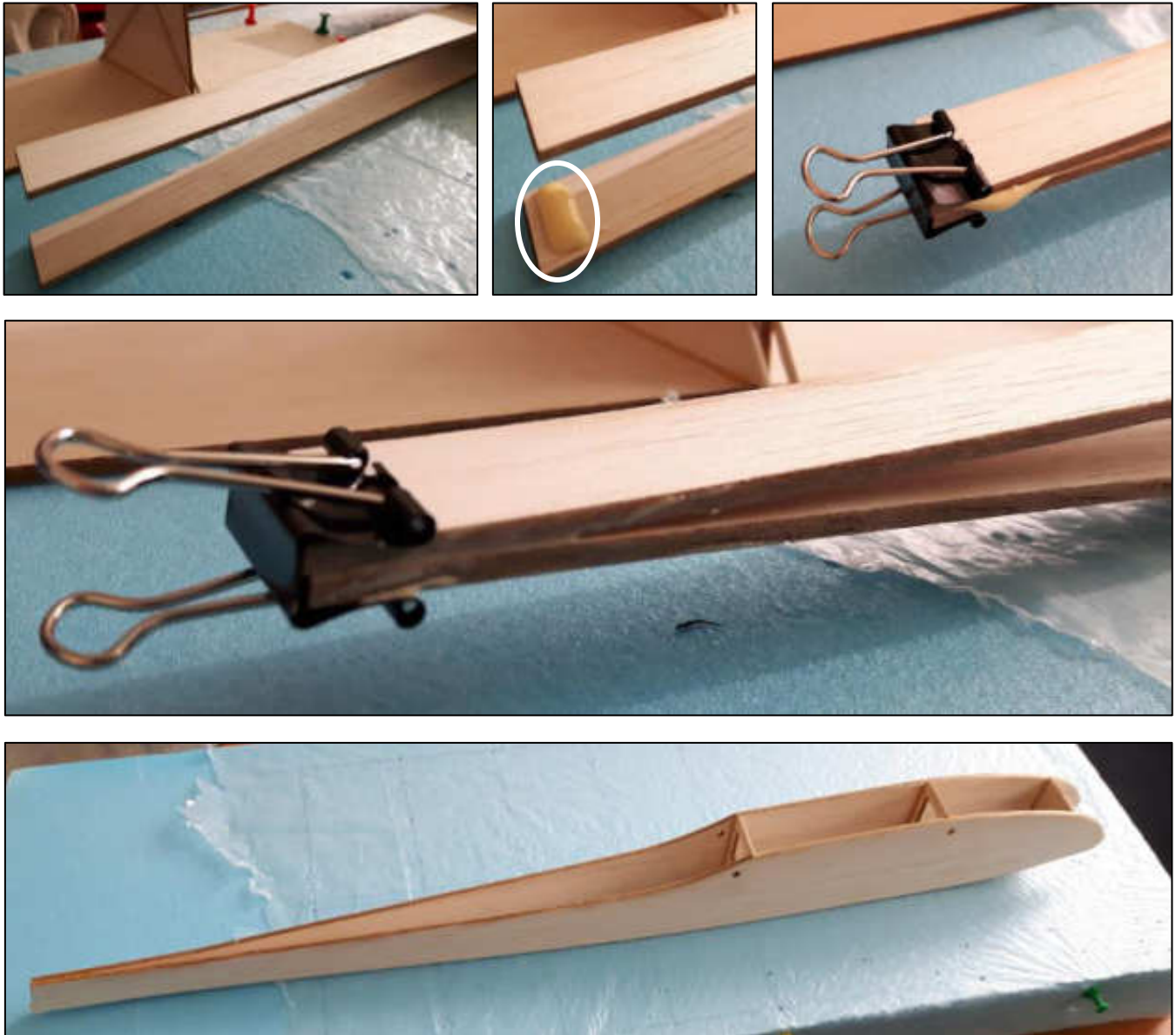
Figure 17: Gluing the tail together.
