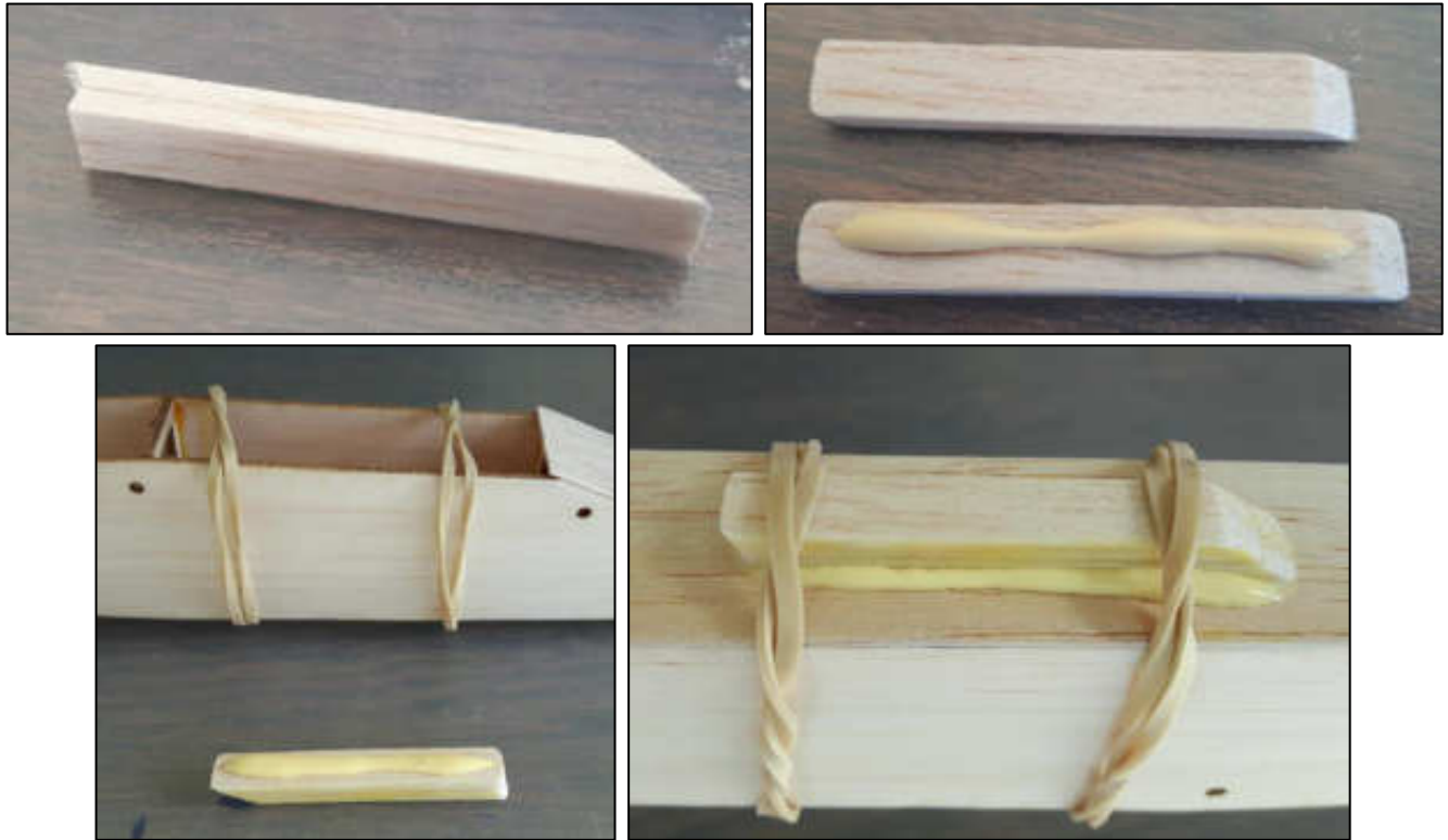
Figure 25: Glue the launch attachment to the fuselage.
