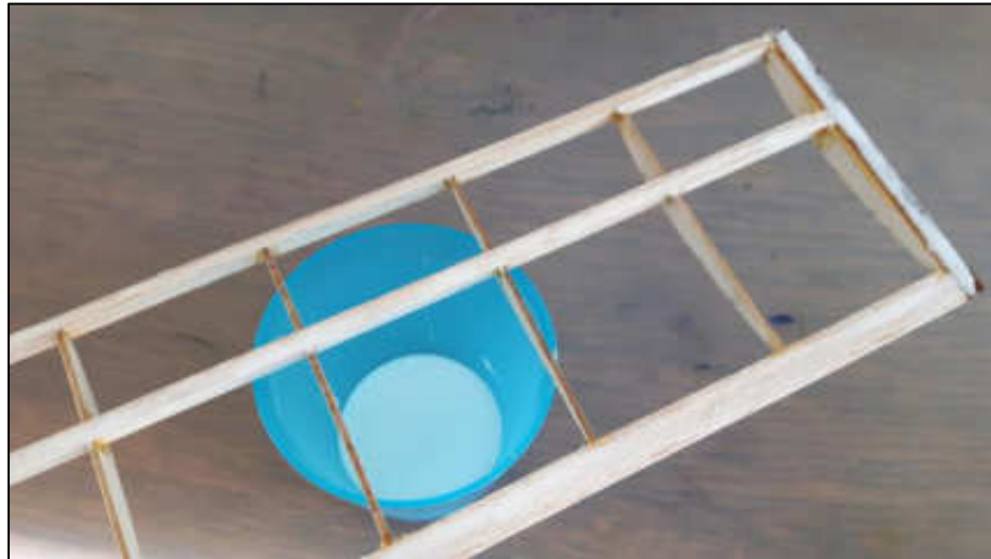
Figure 31: Apply glue to the bottom of the wing.
