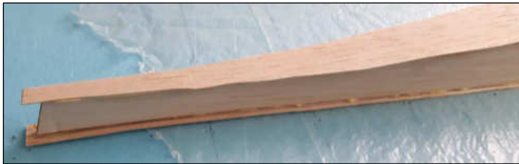
Figure 20: Glue the bottom skin to the fuselage.
