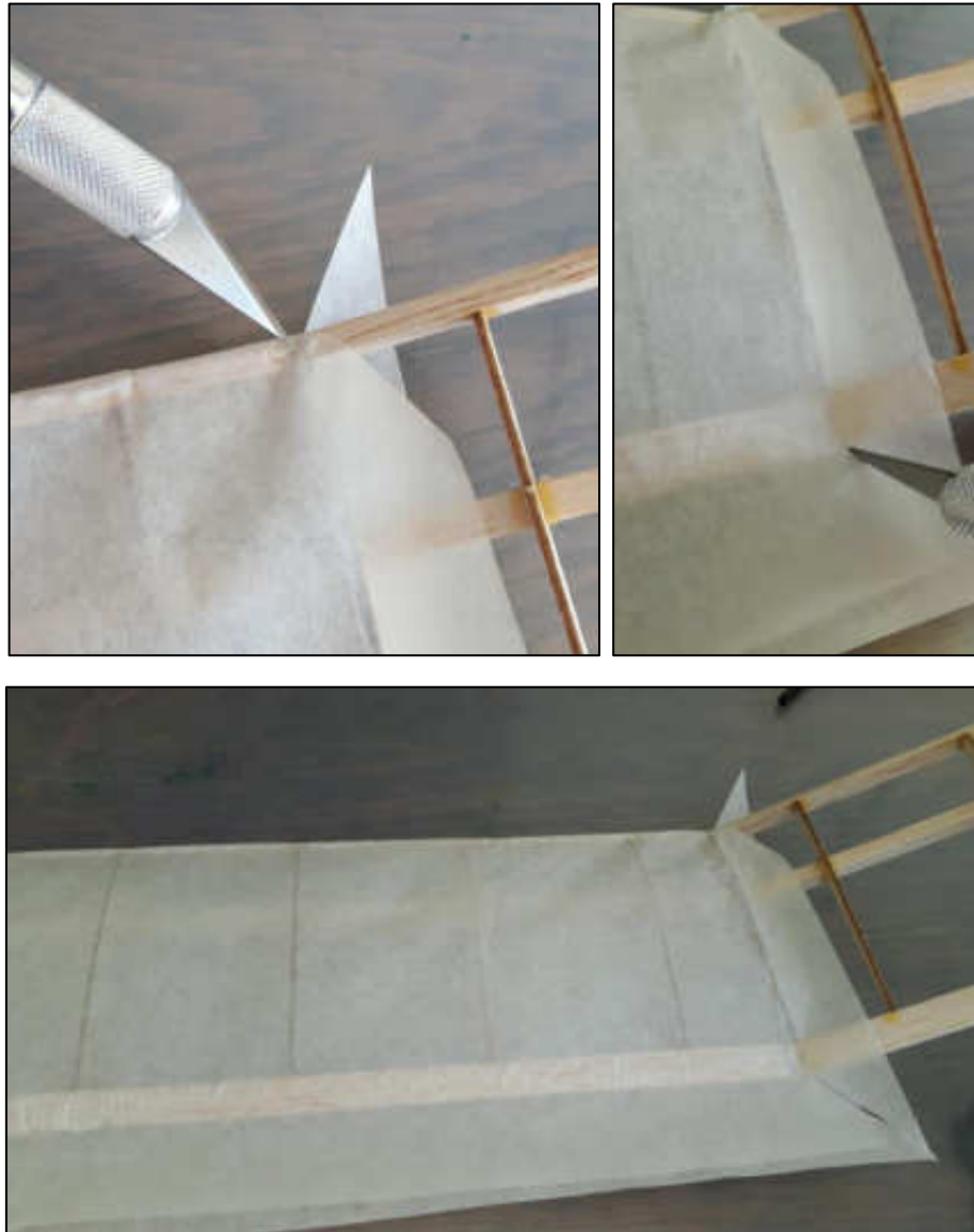
Figure 34: Make cuts to the tissue paper at the wing root.
