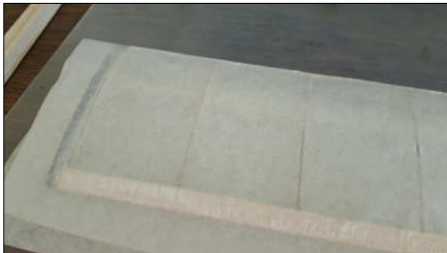
Figure 33: Attaching the wing skin to the wing structure.
