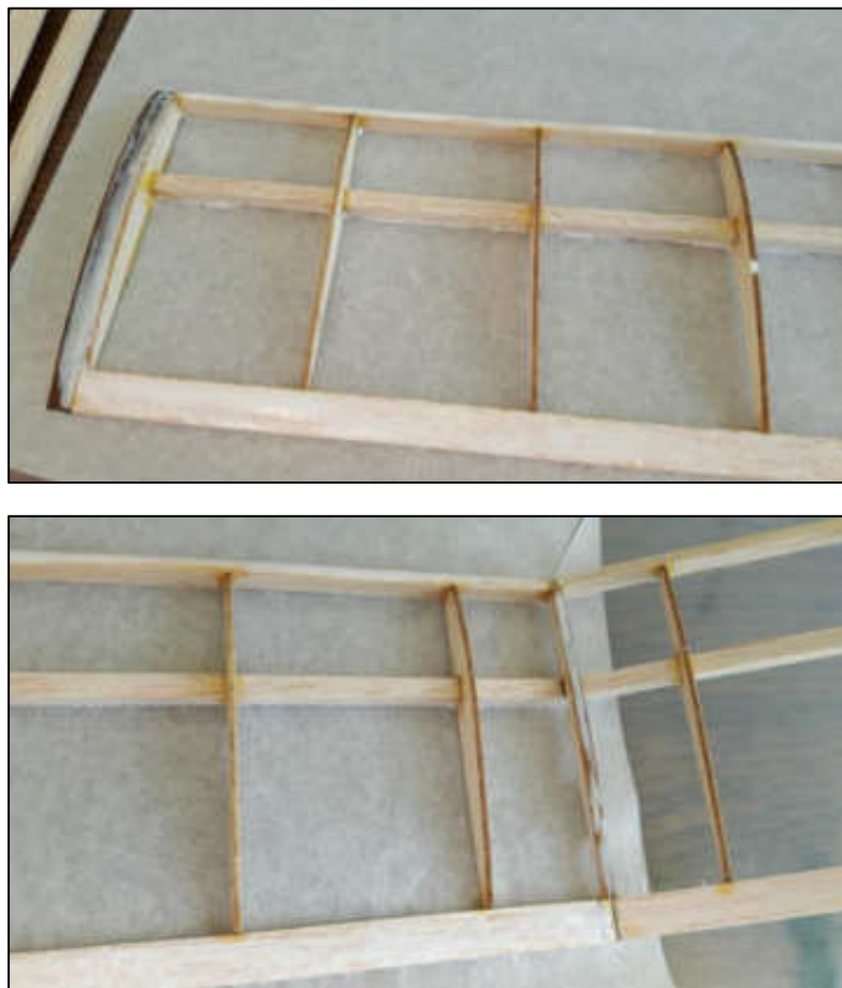
Figure 32: Position the wing on top of the tissue paper.
